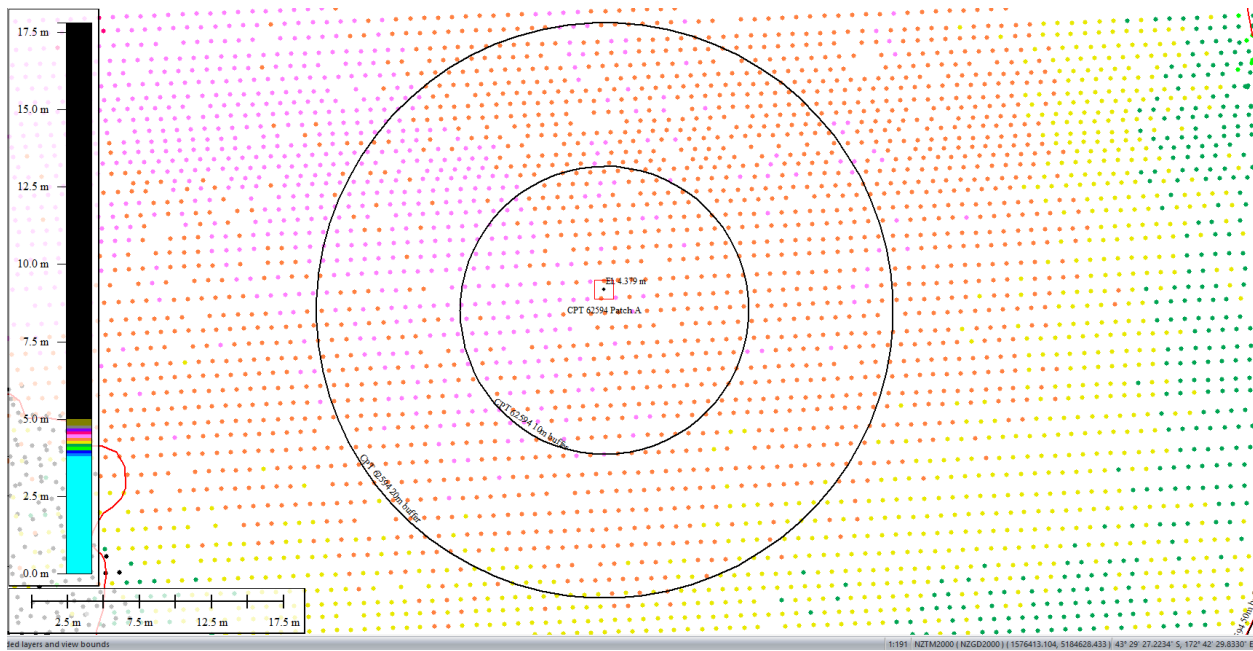
Figure 42: Ground surface elevation averaged over 20-m buffer for Patch A for Sep 5, 2010 LiDAR survey.
